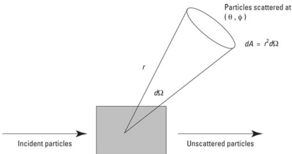
**Figure 12-1:** Scattering from a target.
